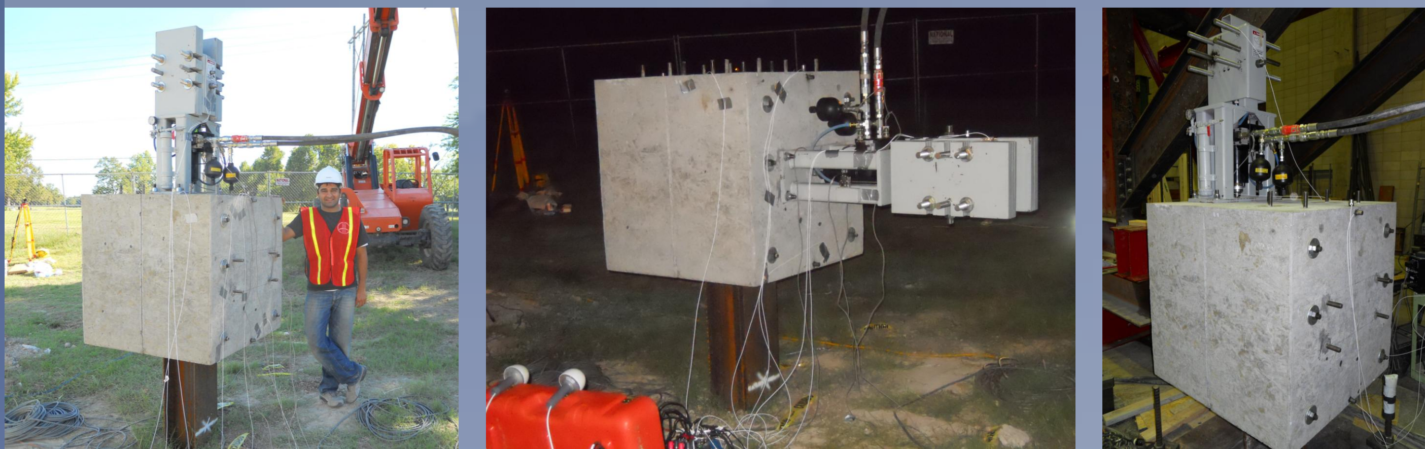
(a) VC test (b) HC test (c) VE test Inertial shaker configurations for the three test types
