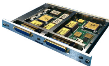
Figure 6.19: The DDC SCS750 computer
