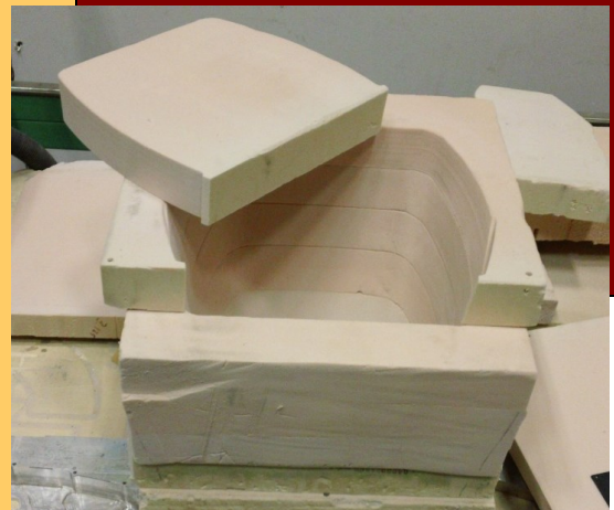
The nose cone is produced one layer at a time by CNC routing the profile out of layers of foam.
