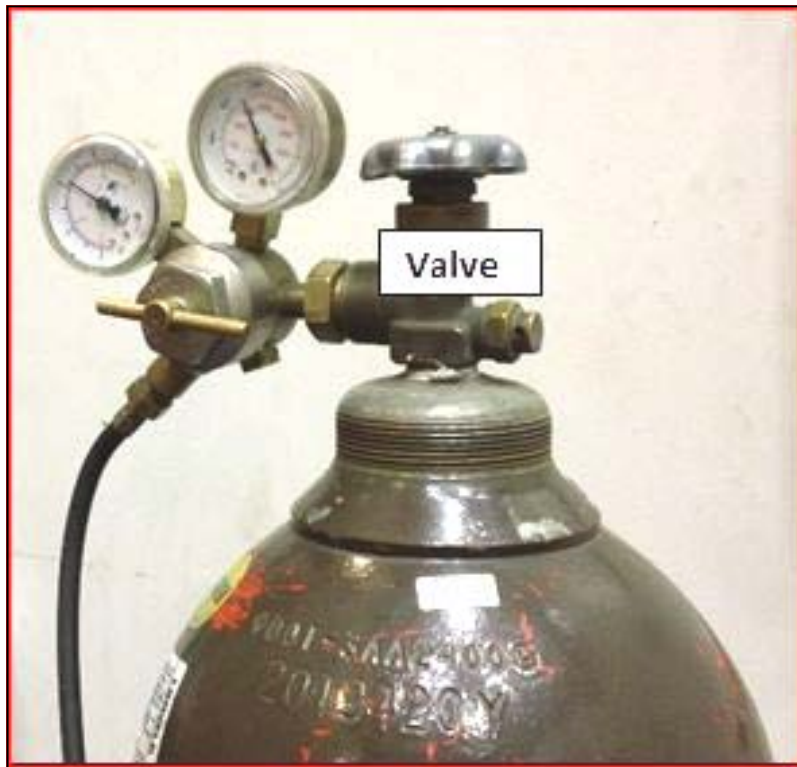
Figure 2N: Tank Valve
