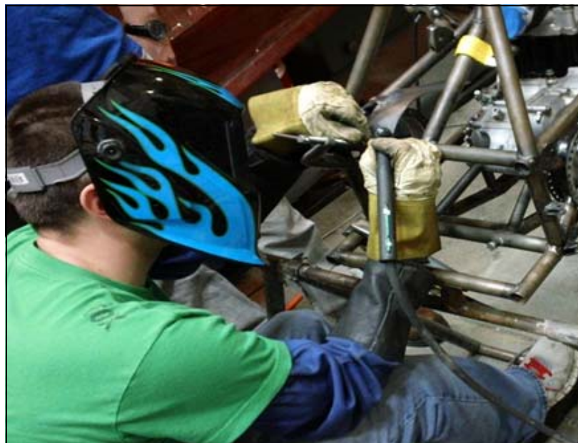
Figure 2M: Proper Welder Safety Gear
