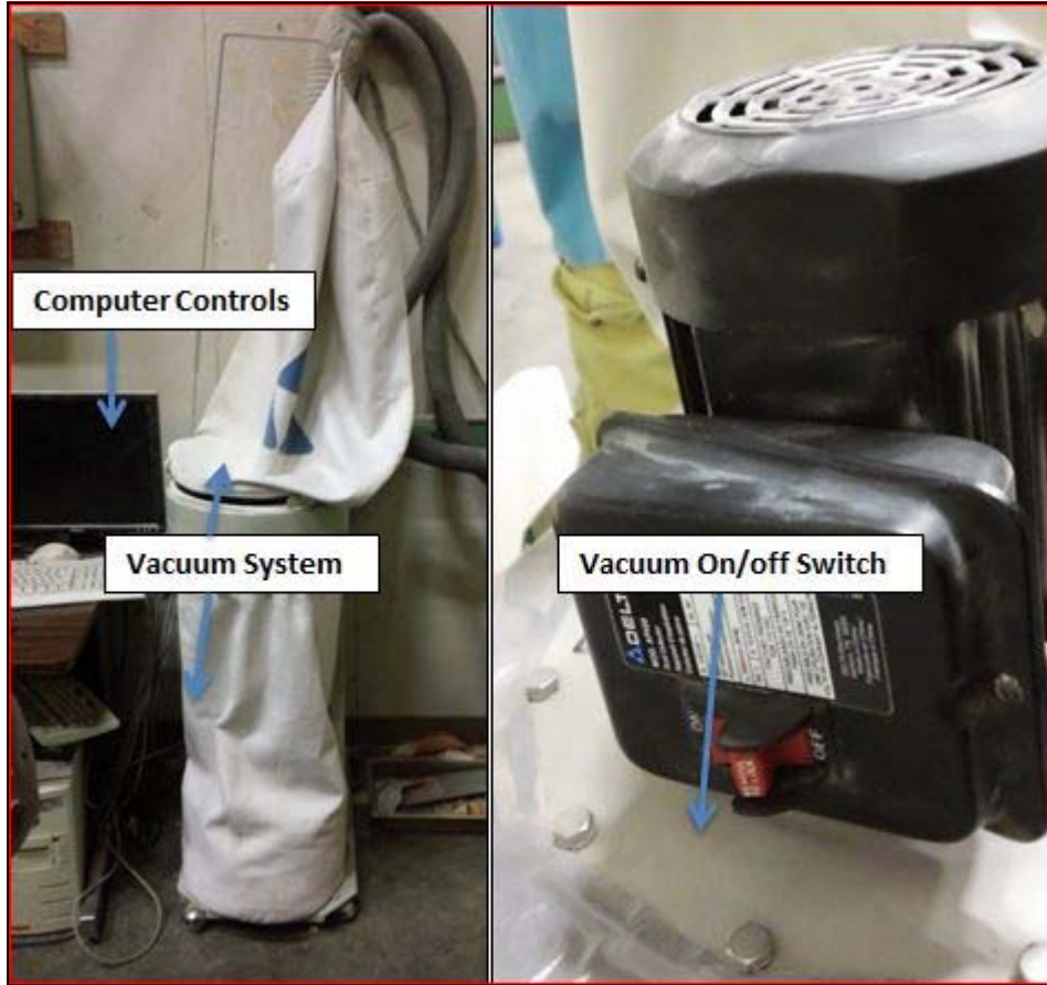
Figure 2I and 2J: CNC Foam Router Vacuum System (Front and Back)
