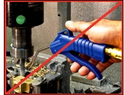
Figure 1I: Don't clean up w/air
